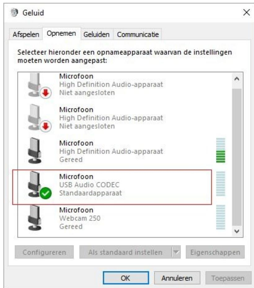
TX (Microphone /recording) to USB Audio Codec
